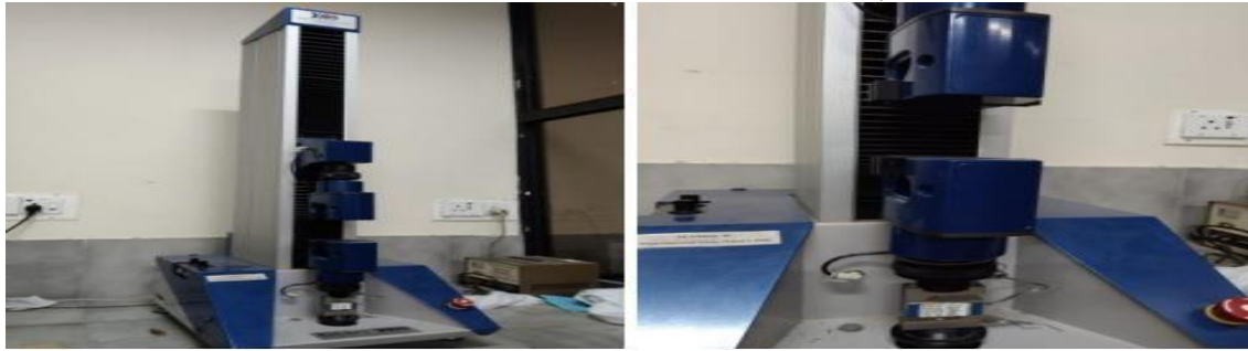
FIGURE 8: TEST FOR TENSILE STRENGTH EQUIPMENT SETUP
