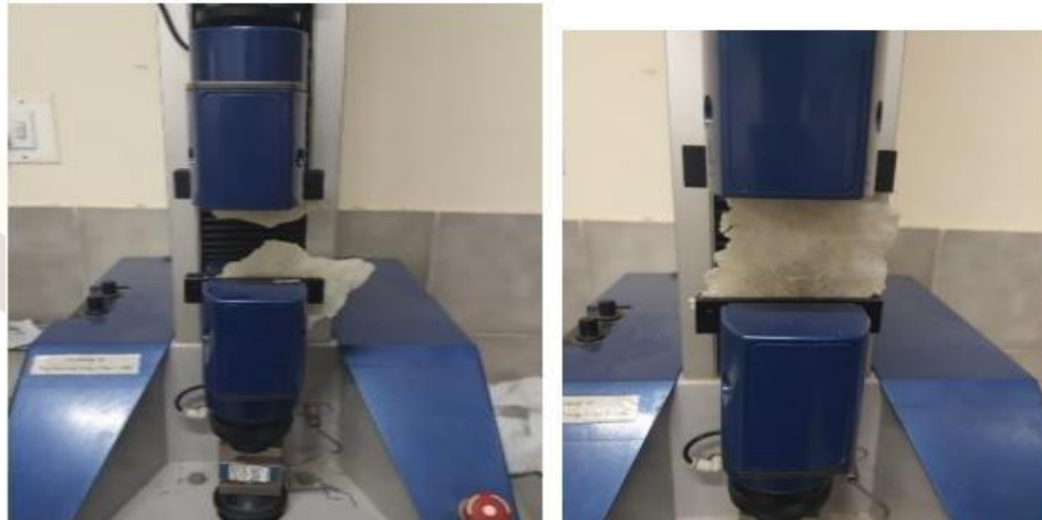
Figure 9: Tensile Testing On Bioplastic Sample Fig (A) Shows Bioplastic Sample And (B) Shows After Breaking Of Bioplastic Sample
